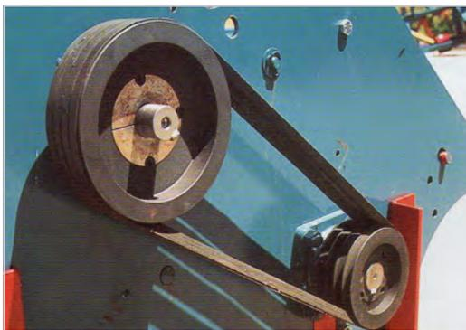
Belt drives lessen the shock loads which mulchers have to endure. Consisting of either 3 or 4 belts, depending on size, they are fitted using taper lock pulleys for ease of maintenance (pictured left). Horsepower requirements largely depend on the terrain and what is being cut, however one should allow approximately 10HP per foot (300mm) of mulcher
