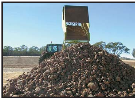
Large 3cu yard hopper on High Rise 8000
