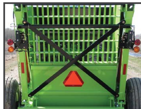
Round bar grated back bucket. High Rise 8000 only
