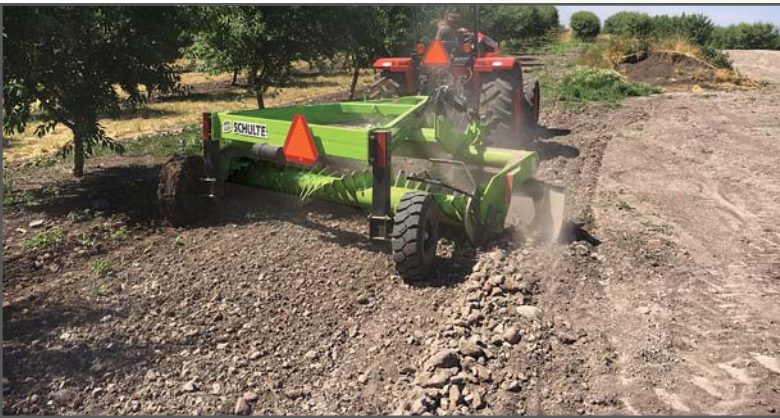
Create clean, uniform rows ready for rock picking
