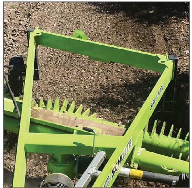
Clean up roots, stumps, chips and other debris from land clearing operations. Breaks lumps and levels the ground
