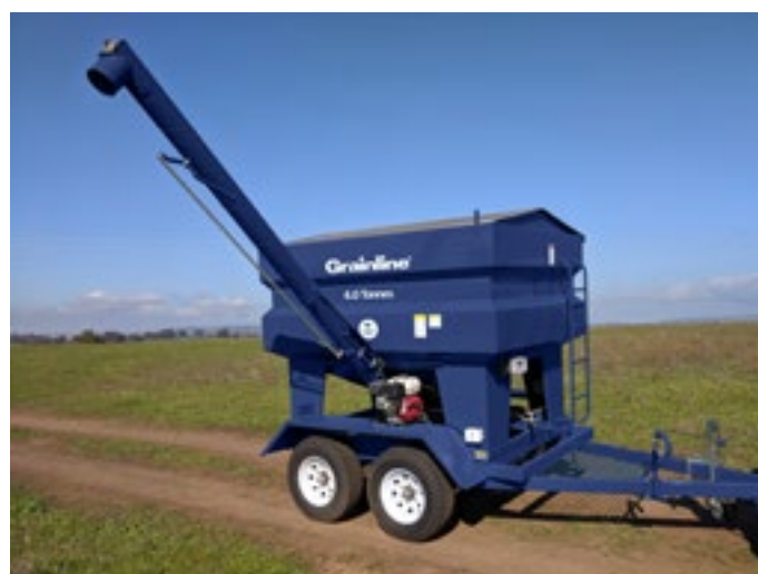
4 Tonne (50 bag) Feed Out Trailer including 3m x 6" Auger
