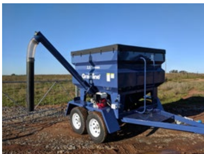
2.5 Tonne (30 bag) Feed Out Trailer including 3m x 5" Auger
